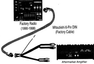
(Low-volt trigger may have to be used when replacing amplifier)
