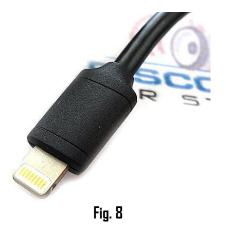
Secure lightning cable in a location away from heat, humidity, moving parts, or sharp metal objects. Damage to lightning plug may occur if subject to abuse.
