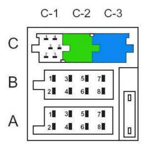
**WARNING:** When installing an auxiliary input adapter to Becker radios, the CD Changer (if present) must be disconnected this includes both the BLUE and GREEN plugs otherwise the "AUX" will not work (no sound).
