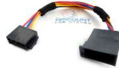
Fig. 5 Power supply harness
