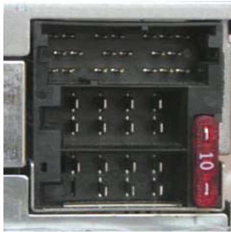
Audi/VW Radio 20/8-pin connectors Fig. 6
