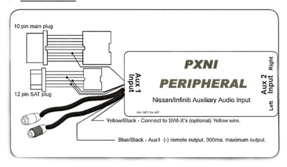
Note to 2007 Maxima & M35: Cut PXNI's red power leads from 10-pin harness and connect to vehicles accessory wire source
