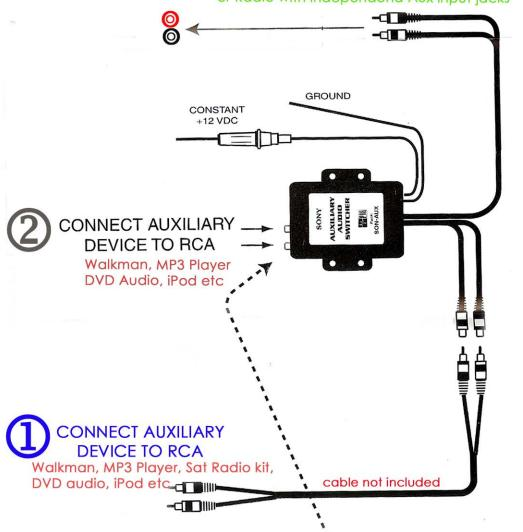
When audio signal is detected from the device on ② the SON-AUX will disconnect the audio from the device on ① and will reconnect with ① if no audio is detected on ②
