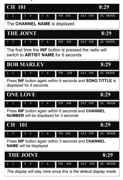
Note: If the **INF** button is not pressed again during any part of the sequence, the display will default to channel name
