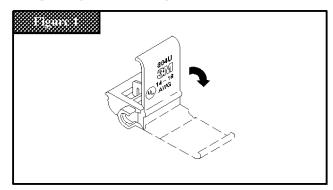
**2.** Place unstripped run wire inside run channel and close hinged side wall (*Figure 2*).
