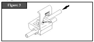
**4.** Hold tool perpendicular to the wire and make the connection by crimping the u–contact down flush with the top of the insulator (*Figure 4*).
