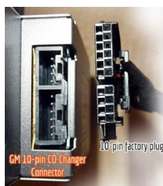
Fig. 5 10-pin socket/10-pin plug
