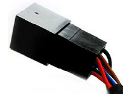
Fig. 5 8-way connector on harness
