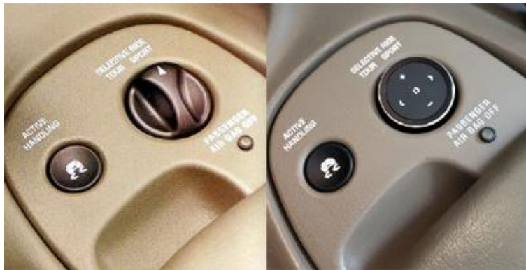
Remote control custom install in place of factory selective drive control switch
