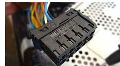
Fig. 4 Factory CD Changer Plug
