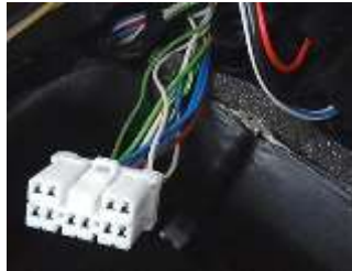
Fig. 18 (shown here 10-pin Female plug)
