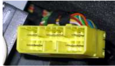
Fig. 19 (shown here 18-pin Male connector)
