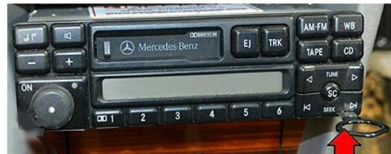
1. Slide tools into radio left and right slots with straight edge facing away until detent position. Withdraw radio by pulling tools. See **Fig. 2**
