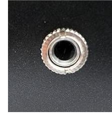
**Warning:** Jack may be left freestanding, but to be mounted, ensure panel is **less than 4mm thick** otherwise shaft may not protrude enough to engage with nut. If necessary, use dremel, sander etc. to thin panel or choose alternate mounting location.
