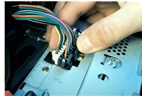
Fig. 1 20-pin radio connector
