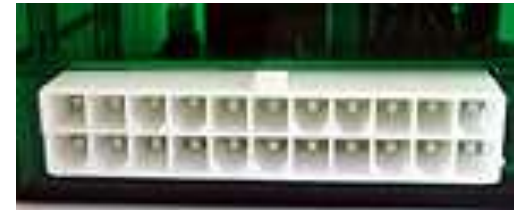
Fig. 4 22-way Molex connector
