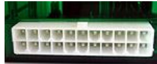
Fig. 4 22-pin Molex connector
